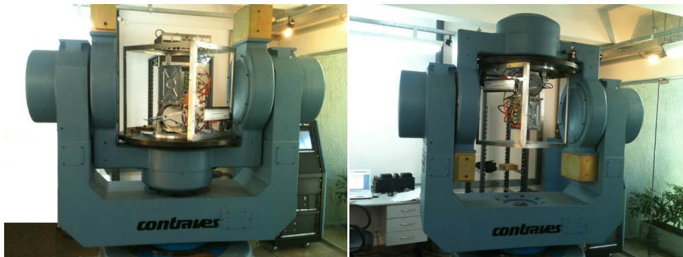
Figure 1. Contraves 3-axis turntable with inner table at 0°(left) and 180° (right)
