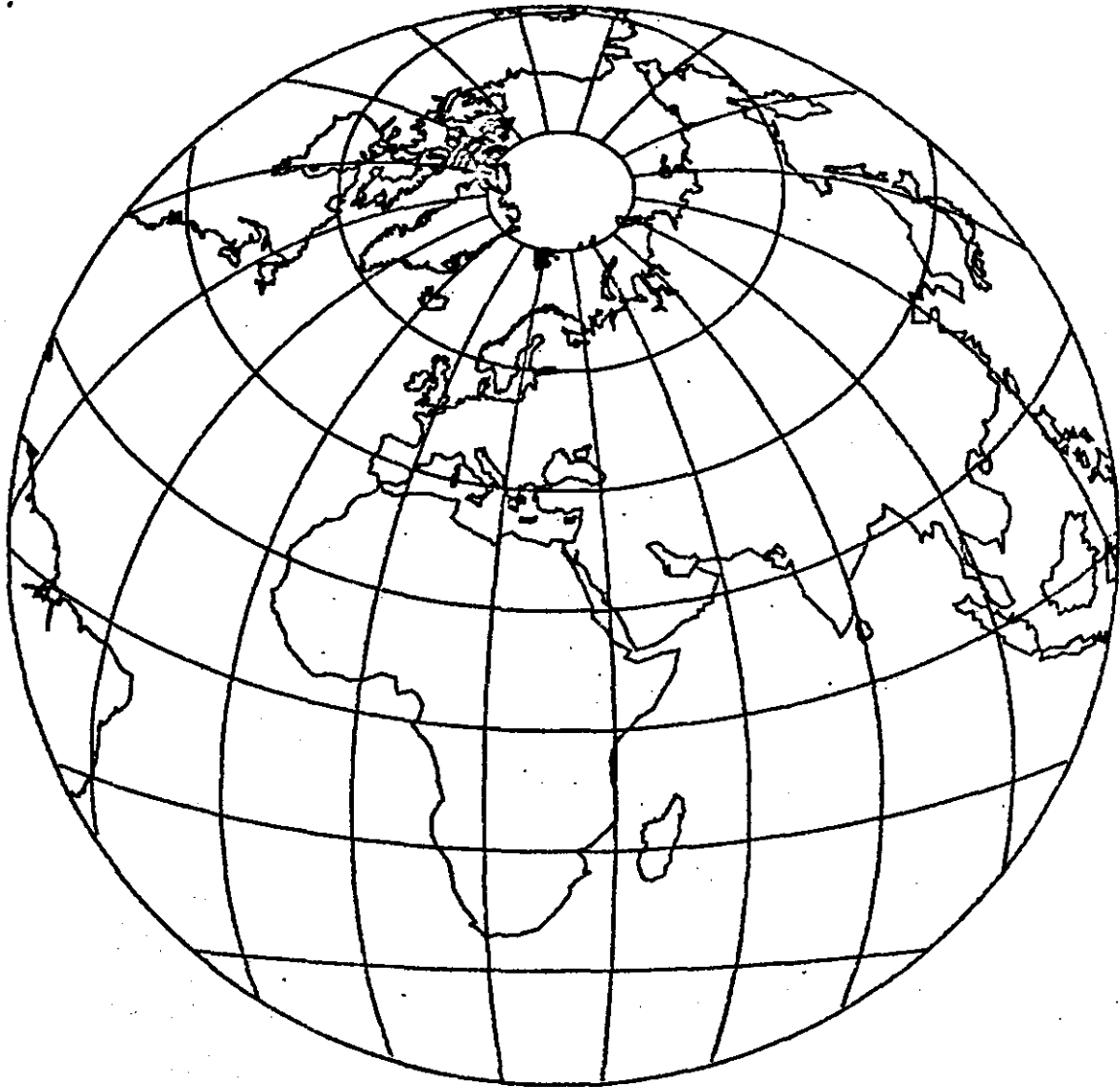
Fig. 23. Azimutal. EI(1)=6, EI(2)=31.5, EI(3)=31, EI(4)=90, EI(11)=51, EI(16)=.15, EI(17)=.97, EI(18)=.88, EI(19)=.13.
